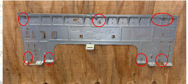
UUT76 wall plate to wall fastener locations
