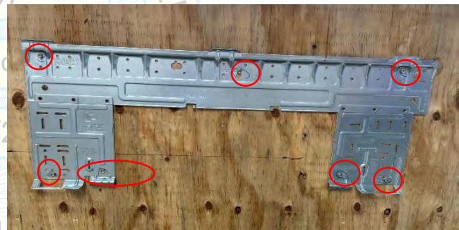
UUT78 wall plate to wall fastener locations
