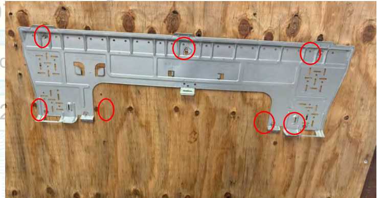
UUT74 wall plate to wall fastener locations
