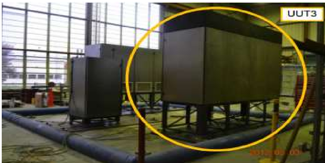
All units were filled with contents and maintained structural integrity and functionality after AC156 test.
