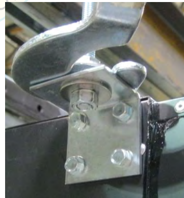
Terminal bracket used for UUT7B tests. Brackets are 12 gage zinc-coated steel attached to unit with four #14 sheet metal screws.
