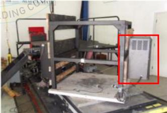
Wall mounted rigid using (8) #12 - 2 1/2" HEX-TEK Screws
