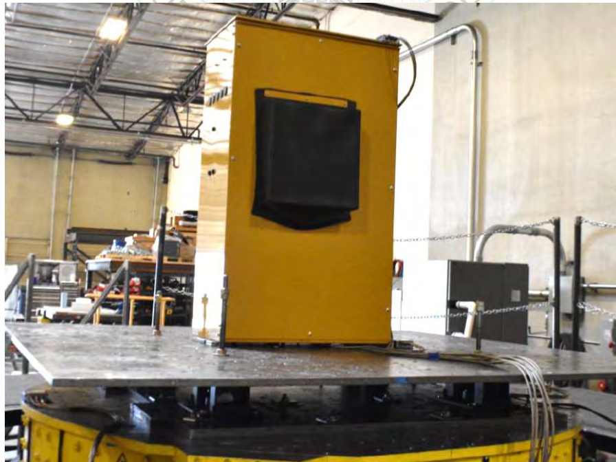
All units were filled with contents and maintained structural integrity and functionality after AC-156 test.
