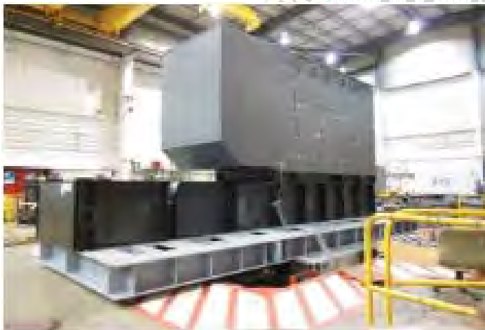
Figure 6C.1: Unit on the shake table
