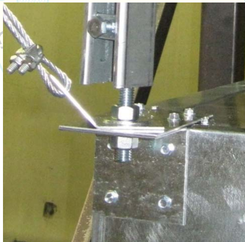
Photograph showing typical mounting for UUT23, UUT26.
