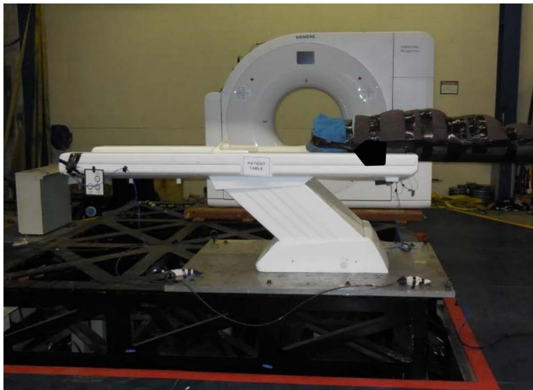
**Manufacturer:** Siemens Healthcare GmbH**Test Location:** Environmental Testing Laboratory**Component:** Patient Table**Test Date:** January 15, 2014**Model Number:** 10355389**Report Number:** SQ35-1401-01 Rev.1**UUT Function:** Motorized patient table**UUT Description:** Component of SOMATOM CT Systems**UUT PROPERTIES**
