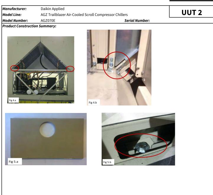
Figures 4.a and 4.b show angle brackets that were installed at each corner of the coil pair, connecting the coil frame to the coil rail (8 brackets total). Brackets were Everbilt 2" corner braces, Model 15267, 12 gage galvanized carbon steel, 0.62" wide.
