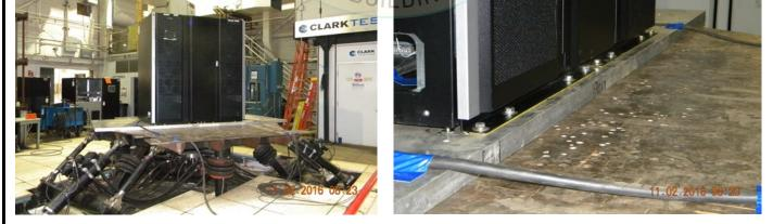
The unit was rigid floor mounted to an Aluminum plate using (16) 1/2" Grade 5 bolts. The Aluminum plate was rigid mounted to the shake table.
