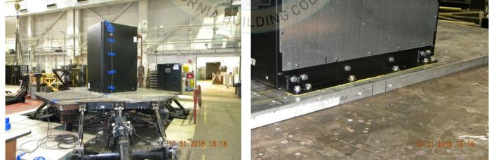
The UUT was rigid mounted to an Aluminum plate using (12) 1/2" Grade 5 bolts. The Aluminum plate was rigid mounted to the shake table.
