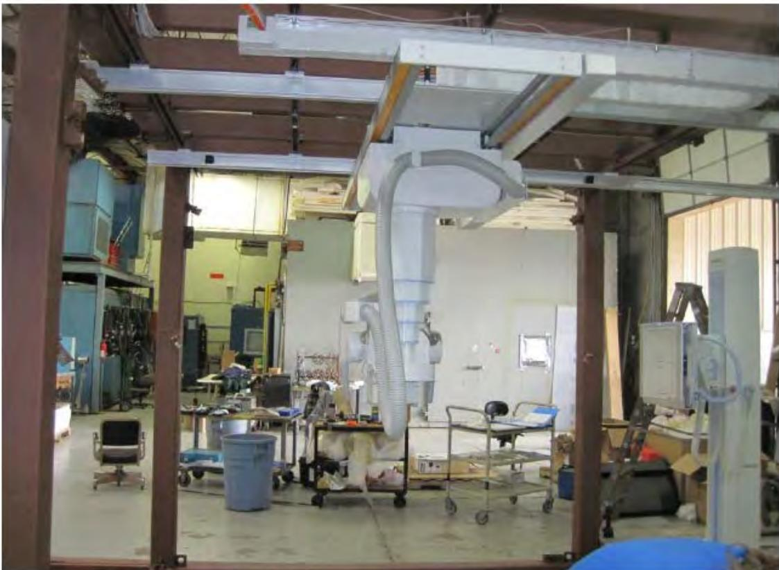
**Manufacturer:** Siemens Healthcare GmbH**Test Location:** Environmental Testing Laboratory**Component:** X-Ray Tube Stand w/ 4m Bridge**Test Date:** March 7 / May 16-17, 2012**Model Number:** 7042224**Report Number:** SQ35-1204-01 Rev. 3**UUT Function:** X-Ray stand, ceiling suspended, for use in radiography imaging, fully automated**UUT Description:** Component of the Luminos dRF System
