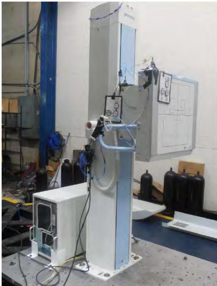
**Manufacturer:** Siemens Healthcare GmbH**Test Location:** Environmental Testing Laboratory**Component:** Tilting Bucky Wall Stand**Test Date:** July 9-12, 2014**Model Number:** 10681704**Report Number:** SQ35-1415-02 Rev. 4**UUT Function:** Radiographic wall stand for X-ray exposures**UUT Description:** Component of the Luminos Agile Max "Seismic Edition" system with Pixium 3543 Ezh detector (10762402)**UUT PROPERTIES**
