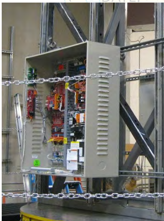
Rigid test setup (UUT3a), cover removed for photograph
