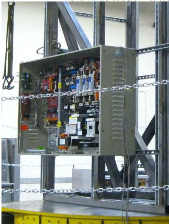
Rigid test setup (UUT1a), cover removed for photograph
