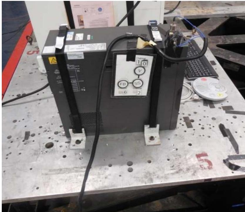
**Manufacturer:** Siemens Healthcare GmbH**Test Location:** Environmental Testing Laboratory**Component:** Image Control System**Test Date:** November 4 - 6, 2014**Model Number:** 10864203**Report Number:** SQ35-1423-01**UUT Function:** Computer for data acquisition, image reconstruction, and processing**UUT Description:** Component of SOMATOM CT Systems
