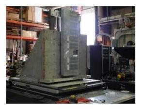
Wall Mounted with (6) 10-32 grade 2 screws with a torque of 30 in/4bs
