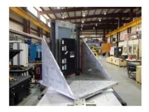
Wall Mounted with (6) 10-32 grade 2 screws with a torque of 30 in / lbs
