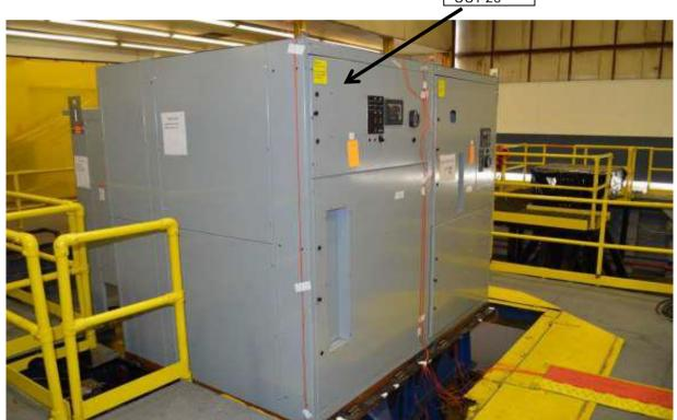
UUT 25 was mounted to a rigid base with (8) 1/2" bolts (Grade 5). The steel frame (carbon steel) was welded to the shake table.
