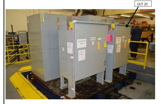
UUT 20 was mounted to a rigid base with (8) 1/2" bolts (Grade 5). The steel frame (carbon steel) was welded to the shake table.
