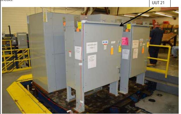
UUT 21 was mounted to a rigid base with (8) 1/2" bolts (Grade 5). The steel frame (carbon steel) was welded to the shake table.
