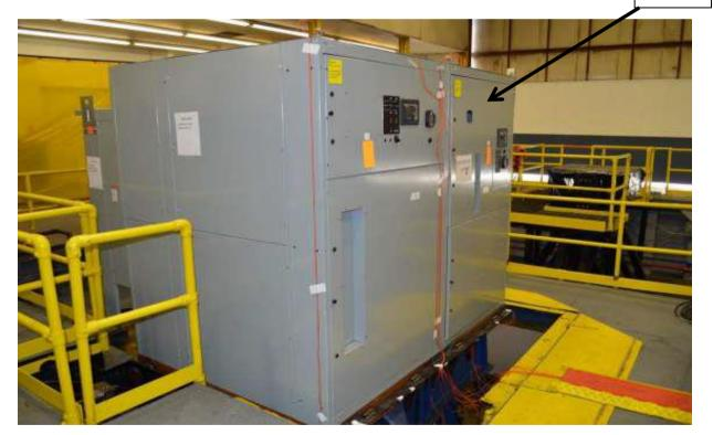
UUT 24 was mounted to a rigid base with (4) 1/2" bolts (Grade 5). The steel frame (carbon steel) was welded to the shake table.
