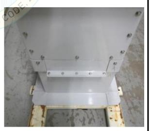
Rigid base mounted on 18" Loren Cook LECQ curb with (20) 3/8" F593 stainless bolts. Curb is welded to test fixture with 2" long welds at 6" O.C. all around.
