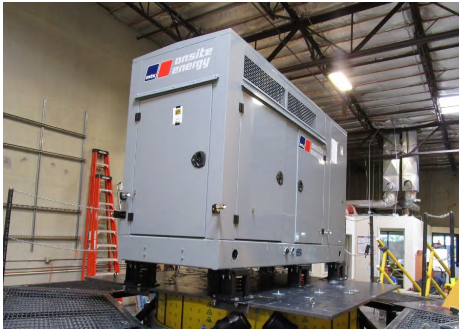
All units were filled with contents and maintained structural integrity and functionality
