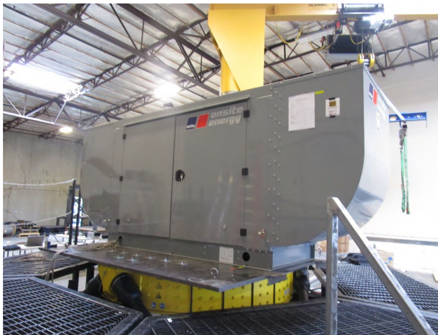
All units were filled with contents and maintained structural integrity and functionality
