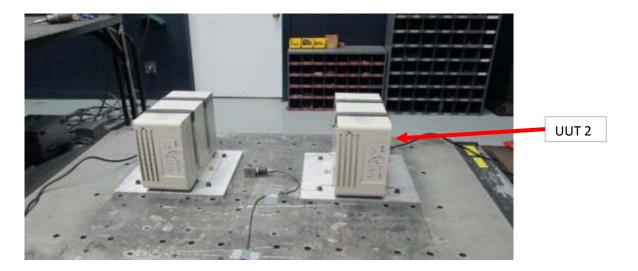
Rigid base mounted to shake table with Falcon Seismic Kit Version #2 and (2) 1/2" grade 8 bolts. Unit maintained structural integrity and remained functional per manufacturer requirement. Contents were included in testing per operating conditions.
