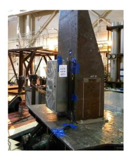
Rigid wall mounted with (4) 7/16" grade 5 cap screws.
