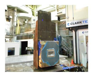
Rigid wall mounted with (4) 7/16" grade 5 cap screws.
