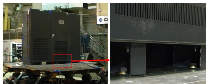
Rigid base mounted with (10) 3/4" Gr. 5 bolts. Unit maintained structural integrity and remained functional per manufacturer requirement. Contents were included in testing per operating conditions.
