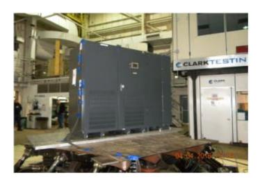
Rigid base mounted with (12) 3/4" Gr. 5 bolts. Unit maintained structural integrity and remained functional per manufacturer requirement. Contents were included in testing per operating conditions.
