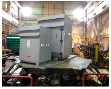
Unit is rigid base mounted to shake table using (4) 5/8" Grade 5 bolts.
