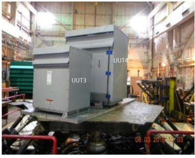
Unit is rigid base mounted to shake table using (4) 1/2" Grade 5 bolts.
