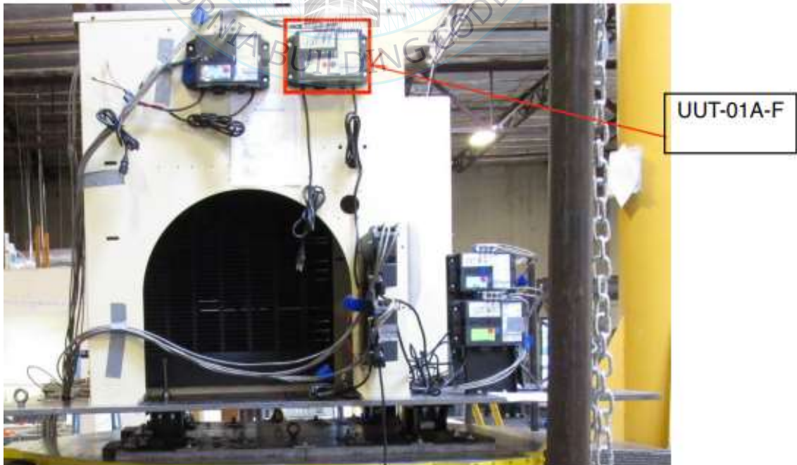
All units were filled with contents and maintained structural integrity and functionality after AC-156 test.
