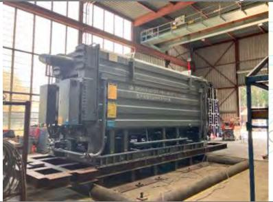
UUT was base mounted - rigid using 5" long 1/4" fillet welds every 3' along four (4) base channels.
