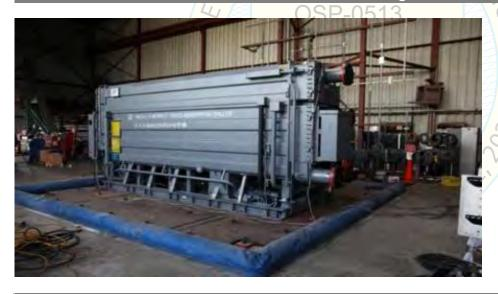
UUT was base mounted - rigid using 2" long 1/4" fillet welds every 12" along four (4) base channels. Unit maintained structural integrity and remained operational per manufacturer requirement following shake table test. All contents were included in the unit per operating conditions.
