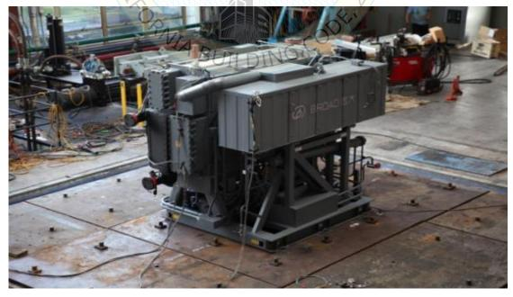
UUT2 was base mounted - rigid using 2" long 1/4" fillet welds every 12" along two (2) base channels.
