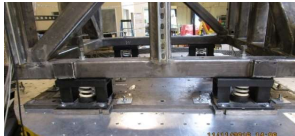
Flexible fixture mounting for UUT6b
