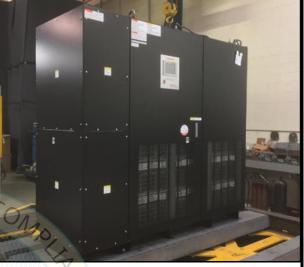
Unit was full of operating content during the shake table test. Unit maintained structural integrity and remained functional per manufacturer requirement after shake table test.
