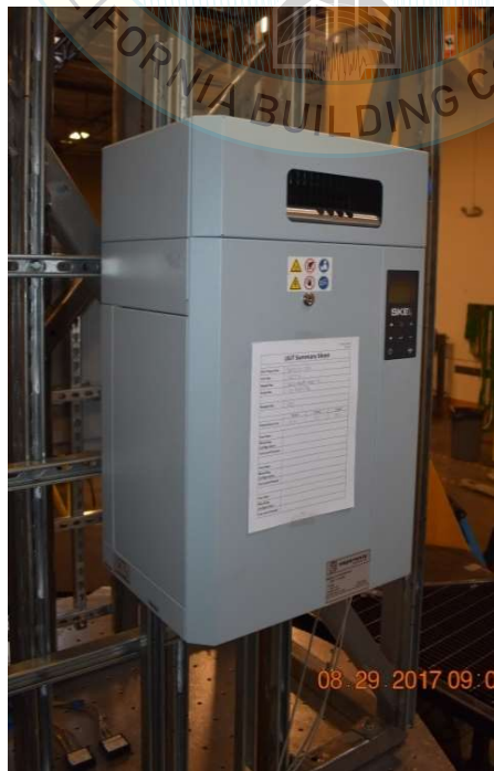
All units were filled with contents and maintained structural integrity and functionality after AC-156 test.
