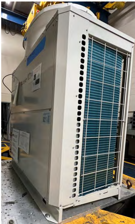
UUT mounted to fixture on shake table with four (4) Grade 8 5/8" bolts with washers.
