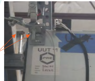
Two Mason SCB/SCBH-0 Braces per hanging rod.
