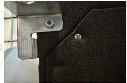
Through bolts M5-Class 8 hex head with washer and nut
