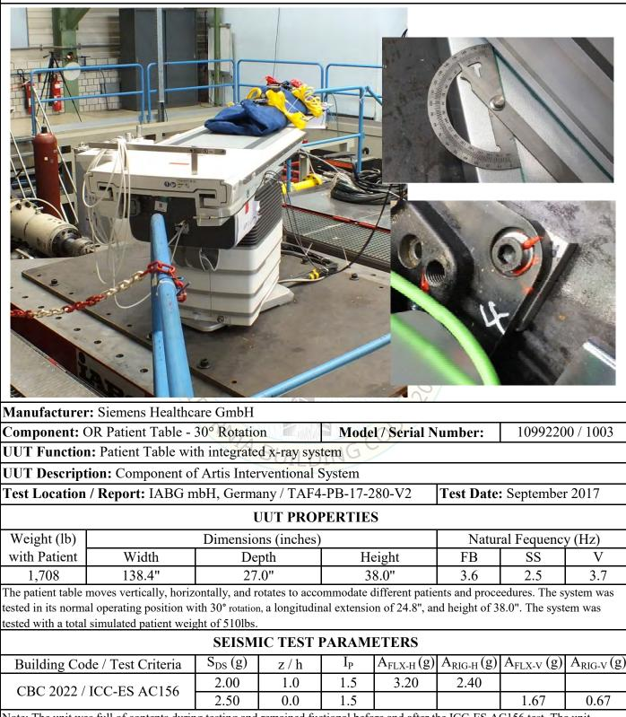
Note: The unit was full of contents during testing and remained fuctional before and after the ICC-ES AC156 test. The unit maintained structural integrity during and after the ICC-ES AC156 Test.
