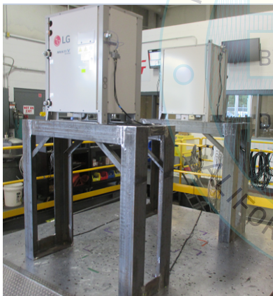
Figure UUT-B1a.1: Unit on the shake table (farthest in photo)
