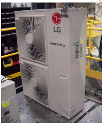
Figure UUT-D2.1: Unit on the shake table
