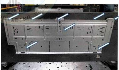
Wall mount plate fastened to wall fixture using eight (8) #10 self-tapping screws. UUT hangs on the wall mount plate and snaps into the wall mount plate.
