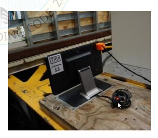
UUT 13 was base mounted - rigid to the table with a custom stainless-steel sheet metal mounting bracket and four #14 x 1-1/2" self-tapping screws. Mounting holes were located at the four corners of the bracket. Four M4-0.7 x 6mm Class 10.9 button head screws were used to secure UUT 13 to the bracket.
