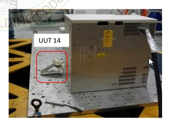
The console bracket base of UUT 14 was mounted to the shake table with two 1" x 4" strips of 3M Dual Lock Reclosable Fastener (P/N TB3550). The mini console of UUT 14 was attached to the bracket with one 1" x 3" strip of 3M Dual Lock Reclosable Fastener. Unit maintained structural integrity and remained functional per manufacturer requirement after shake table test. Contents were included in testing per operating conditions.
