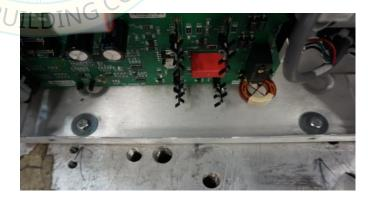
UUT 5 was base mounted – rigid to the table with four 1/4"-20 x 1-1/2" Grade 5 bolts and flat washers. Mounting holes were located inside the generator housing at each corner.
