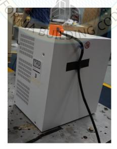
UUT 3 was base mounted - rigid to the table with three 1/4"-20 x 1-1/2" Grade 5 bolts and flat washers. Mounting holes were located inside the generator housing at each corner.
