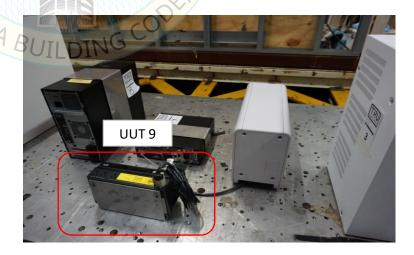
UUT 9 was base mounted – rigid to the table with a custom stainless-steel sheet metal mounting bracket and four #14 x 1-1/2" self-tapping screws. Mounting holes were located at the four corners of the bracket. Four M4-0.7 x 6mm Class 10.9 button head screws were used to secure UUT 9 to the bracket.
