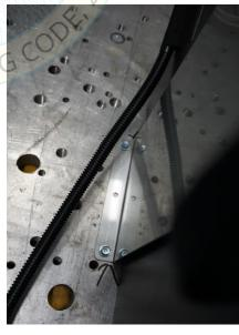
UUT 8 was base mounted – rigid to the table with a custom stainless-steel sheet metal mounting bracket and four #14 x 1-1/2" self-tapping screws. Mounting holes were located at the four corners of the bracket.
