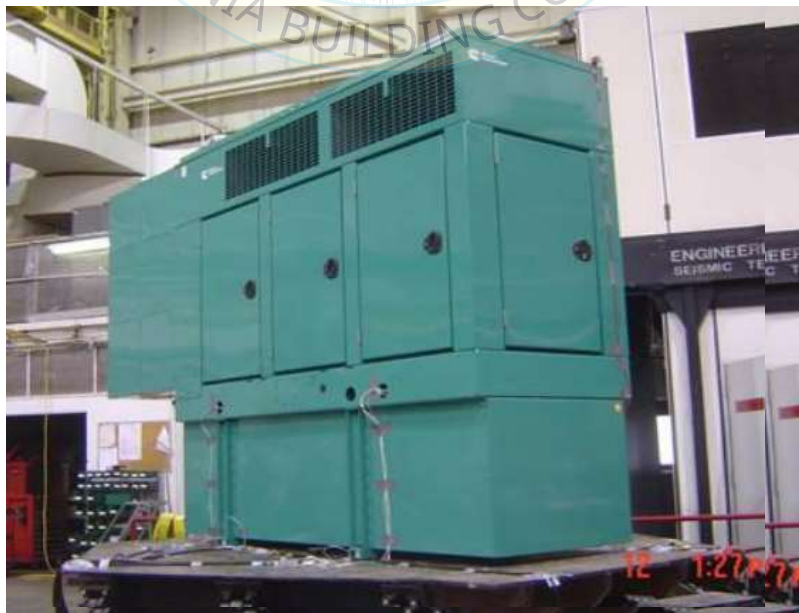
All units maintained structural integrity and functionality after AC-156 test.
