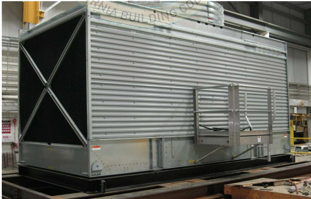
All units were filled with contents and maintained structural integrity and functionality
