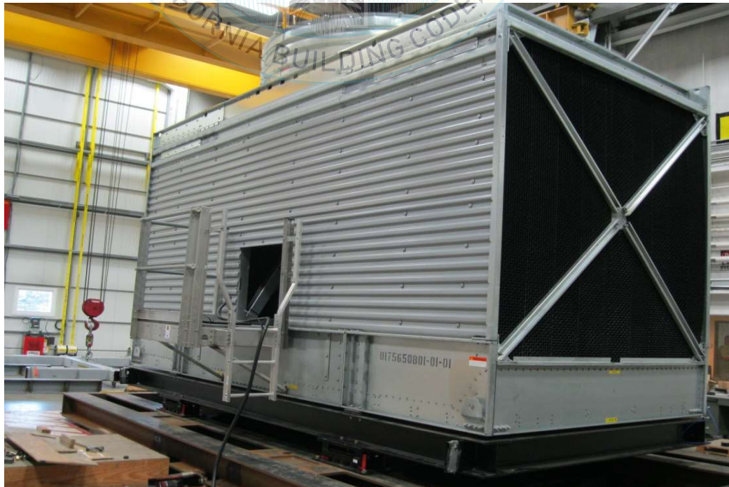
All units were filled with contents and maintained structural integrity and functionality
