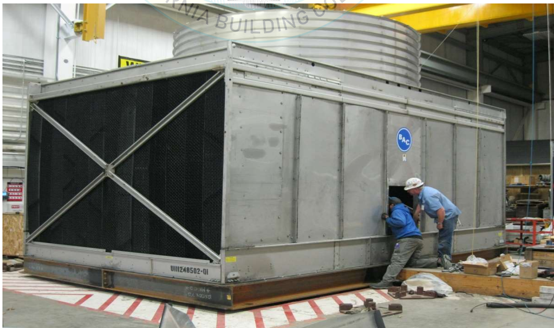
All units were filled with contents and maintained structural integrity and functionality
