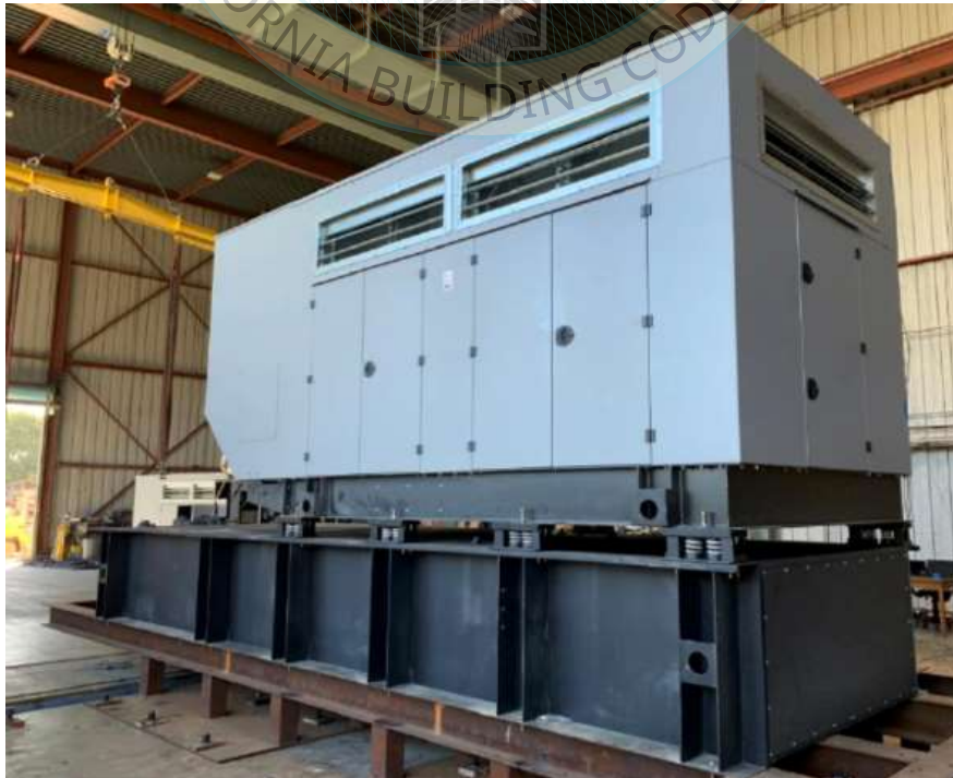
All units were filled with contents and maintained structural integrity and functionality after AC-156 test.
