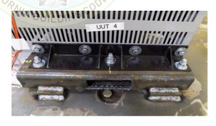
Unit was base mounted-rigid with six (6) 3/8"-16 grade 2 bolts, flat washers and lock washer. Mounting bracket PN: 196BKD001 was used at the front and back of the unit.
