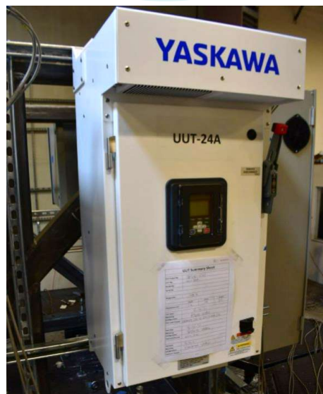
All units were filled with contents and maintained structural integrity and functionality after AC-156 test.
