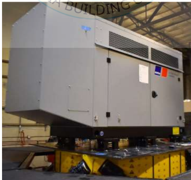
All units were filled with contents and maintained structural integrity and functionality after AC-156 test.
