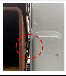
UUT2 was wall mounted - rigid to a wall fixture. The mounting brackets (2 large [Serial No.: 2100303422P7]) were mounted to the wall fixture using eleven (11) 5/16" Grade 5 bolts and lock washers.
