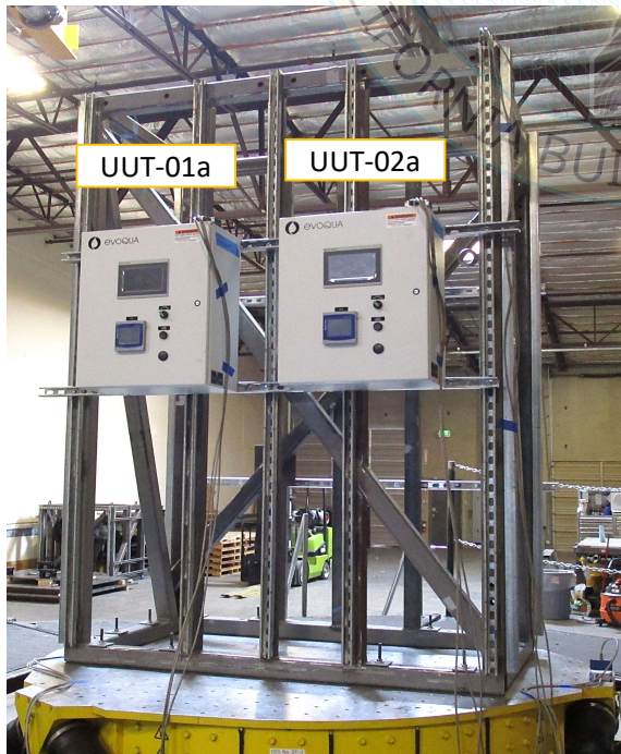
Figure 1. Photograph of UUT-01a and UUT-02a, rigid configuration
