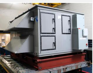
shake table test. Unit maintained structural integrity and remained functional per manufacturer requirement after shake table test.
