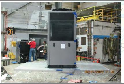
UUT 1 was mounted to seismic table using a total of four (4) 3/8"-16 SAE grade 5 hex bolts with washers and lock washers and torqued to 25ft-lb. One bolts was used per each angle brackets.
