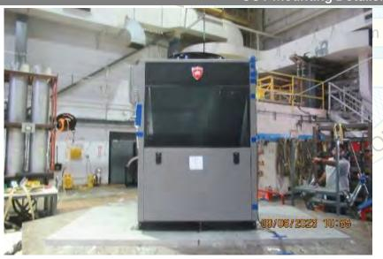
UUT 2 was mounted to seismic table using a total of four (4) 3/8"-16 SAE grade 5 hex bolts with washers and lock washers and torqued to 25ft-lb. One bolts was used per each angle.
