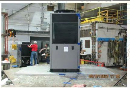
UUT 1 was mounted to seismic table using a total of four (4) 3/8"-16 SAE grade 5 hex bolts with washers and lock washers and torqued to 25ft-lb. One bolt was used per angle bracket. Bracket details on next page.
