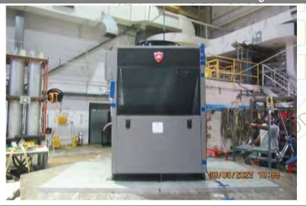
UUT 2 was mounted to seismic table using a total of four (4) 3/8"-16 SAE grade 5 hex bolts with washers and lock washers and torqued to 25ft-lb. One bolt was used per angle.
