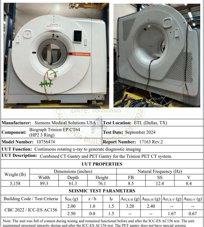
certification and is not included as certified component. The certification applies only to the components of the CT system.
