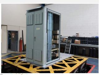
Mounting: Unit was rigid base mounted to the fixture using (4) total 1/2-in Grade 5 bolts through the anchor plates. Anchor plates attach to the internal frame corner bracket using (6) 1/4-in screws per corner and include a welded spacer plate to eliminate anchor bolt bending.
