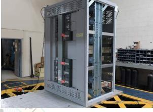
Importance Factor,  $I_P = 1.5$ : Unit was full of operating content during the shake table test. Unit maintained structural integrity and remained functional per manufacturer requirement after shake table test.
