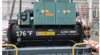
Mounting: Base mounted neoprene vibration isolated. UUT was mounted on (4) Mason neoprene pad assemblies (P/N 028-12849-
