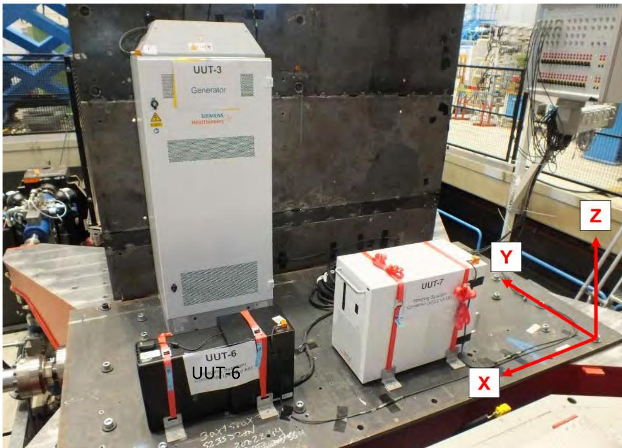
**Manufacturer:** Siemens Healthcare GmbH**Test Location:** IABG - Munich, Germany**Component:** IS PC Container / pS22 PIKE PC**Test Date:** Feb 26, 2025**Model Number:** 11688629 / 11513997**Report Number:** TA-B006468\_V1**UUT Function:** Computer for data acquisition, image reconstruction, and processing**UUT Description:** Component of YSIO X.pree and LUMINOS Q.namix T/R X-Ray and Fluoroscopy Systems**UUT PROPERTIES**
