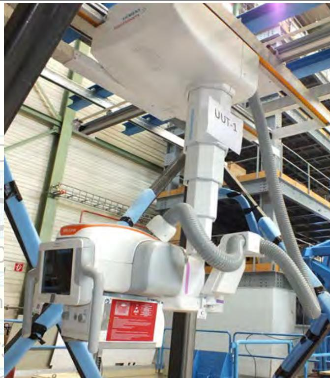
**Manufacturer:** Siemens Healthcare GmbH**Test Location:** IABG - Munich, Germany**Component:** Tube Stand 3D V GB semi-motor / Carriage 3D V 3m **Test Date:** July 29-30, 2024**Model Number:** 11565240 (stand) / 07042133 (carriage) **Report Number:** TA-B-005196-V1**UUT Function:** X-Ray stand, ceiling suspended, for use in radiography imaging, fully automated**UUT Description:** Component of YSIO X.pree and LUMINOS Q.namix T/R X-Ray and Fluoroscopy Systems**UUT PROPERTIES**
