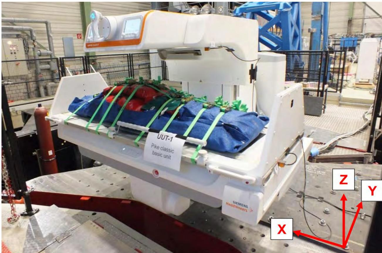
**Manufacturer:** Siemens Healthcare GmbH**Test Location:** IABG - Munich, Germany**Component:** PIKE Classic dTF Table**Test Date:** Feb 26, 2025**Model Number:** 11564199**Report Number:** TA-B-006466\_V1**UUT Function:** Motorized patient table for support and positioning for image acquisition**UUT Description:** Component of YSIO X.pree and LUMINOS Q.namix T/R X-Ray and Fluoroscopy Systems**UUT PROPERTIES**
