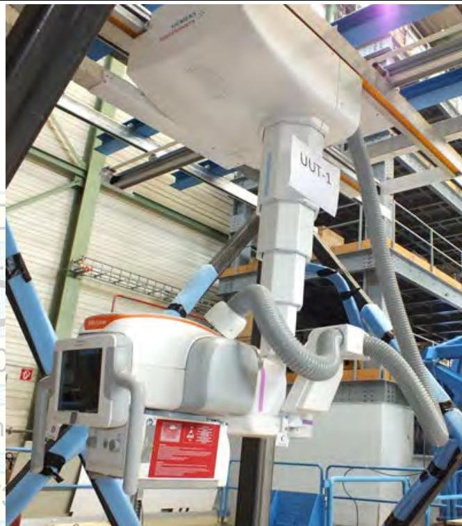
**Manufacturer:** Siemens Healthcare GmbH**Test Location:** IABG - Munich, Germany**Component:** Tube Stand 3D V SF / Carriage 3D 3m SF motorized**Test Date:** Sept 21-23, 2020**Model Number:** 07042125 (stand) / 07042091 (carriage)**Report Number:** TAB3-PB-20-134-V1**UUT Function:** X-Ray stand, ceiling suspended, for use in radiography imaging, fully automated**UUT Description:** Component of YSIO X.pree and LUMINOS Q.namix T/R X-Ray and Fluoroscopy Systems**UUT PROPERTIES**
