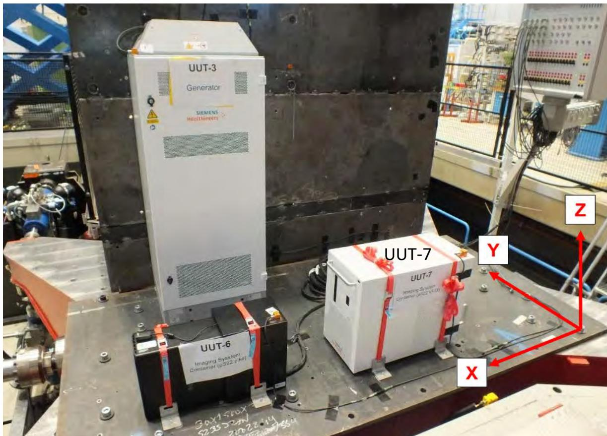
**Manufacturer:** Siemens Healthcare GmbH**Test Location:** IABG - Munich, Germany**Component:** IS PC Container / pS22-VF1X FluoroFD PC**Test Date:** Feb 26, 2025**Model Number:** 11688800 / 11513968**Report Number:** TA-B006468\_V1**UUT Function:** Computer for data acquisition, image reconstruction, and processing**UUT Description:** Component of YSIO X.pree and LUMINOS Q.namix T/R X-Ray and Fluoroscopy Systems**UUT PROPERTIES**
