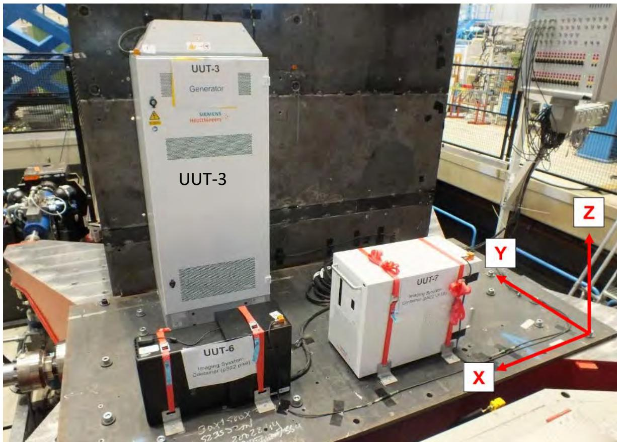
**Manufacturer:** Siemens Healthcare GmbH**Test Location:** IABG - Munich, Germany**Component:** Generator Polydoros RFX (UG-F80-2WP)**Test Date:** Feb 26, 2025**Model Number:** 11011022 / 11011806**Report Number:** TA-B006468\_V1**UUT Function:** Regulate voltage, power distribution**UUT Description:** Component of YSIO X.pree and LUMINOS Q.namix T/R X-Ray and Fluoroscopy Systems**UUT PROPERTIES**
