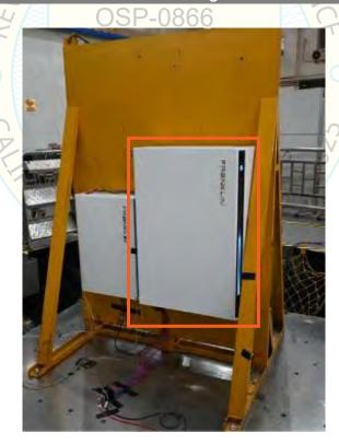
UUT was rigid wall mounted using (4) Grade 8.8 M6 bolts.
