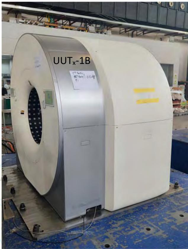
**Manufacturer:** United Imaging Healthcare**Test Location:** EETI (Suzhou, CHINA)**Component:** uMI Panorama 35 PET**Test Date:** June 27, 2023**Model Number:** 78011741**Report Number:** 1340-07**UUT Function:** Use of small amounts of radioactive material to generate diagnostic imaging**UUT Description:** Component of the uMI Panorama GS PET-CT systems**UUT PROPERTIES**
