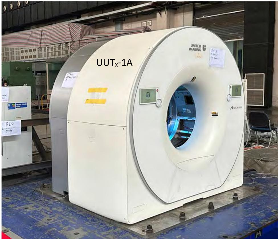
**Manufacturer:** United Imaging Healthcare**Test Location:** EETI (Suzhou, CHINA)**Component:** U80P Panorama CT**Test Date:** June 27, 2023**Model Number:** 78006465**Report Number:** 1340-07**UUT Function:** Continuous rotating x-ray to generate diagnostic imaging**UUT Description:** Component of the uMI Panorama GS PET-CT systems**UUT PROPERTIES**
