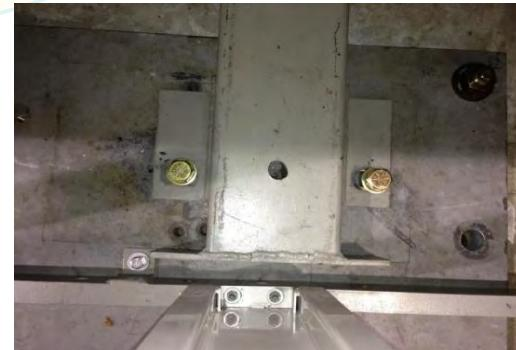
UUT4 was base mounted - rigid to the test fixture using eight (8) 1/2" Grade 5 bolts for the enclosure and twelve (12) 1" Grade 5 bolts for the transformer assembly. Unit maintained structural integrity and remained functional per manufacturer requirement after shake table test. Contents were included in testing per operating conditions.
