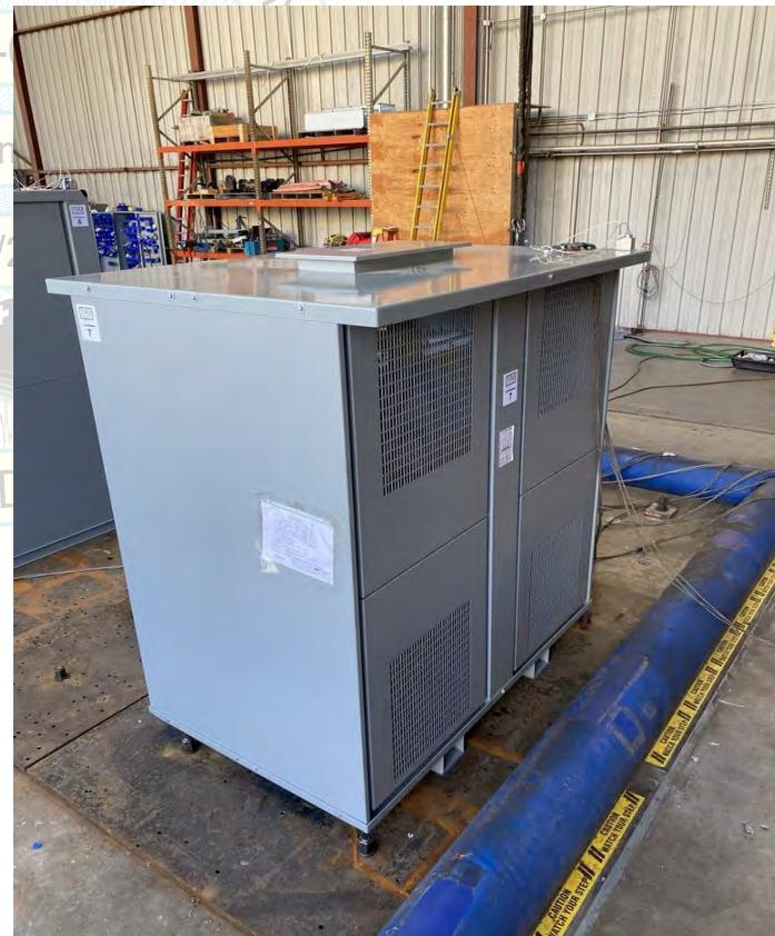
UUT7 was base mounted - rigid to the test fixture using four (4) 7/8" Grade 8 bolts and flat washers.
